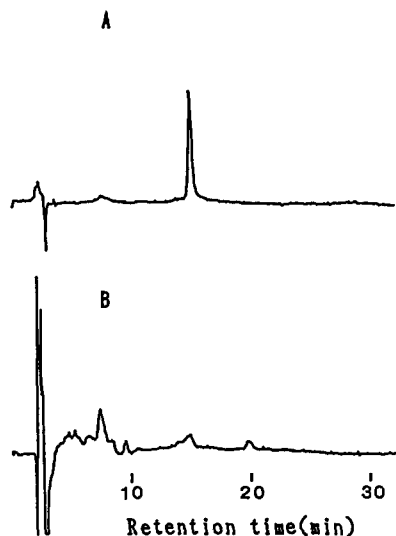
Fig. 6. High-performance liquid chromatograms. (A) Nitroxynil standard; (B) nitroxynil in raw milk sample. HPLC conditions: column, LiChrospher 100 RP-18 (5 \mu m, 250 \times 4 mm I.D.); mobile phase, acetonitrile-0.05 M potassium dihydrogenphosphate (20:80, v/v), pH 4.0; flow-rate, 1 ml/min at 40°C. Coulometric detector: guard cell, -0.7 V; detector 1, -0.7 V; detector 2, +0.7 V; gain, 10 \times 40; response time, 10 s.
